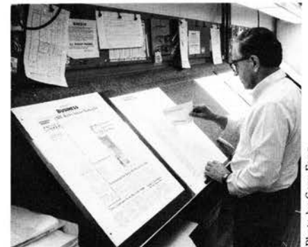
Figure 2.8 Production worker pasting up type on a makeup sheet
