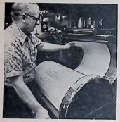
The mat is then sent to the stereo foundry where it is put in a machine which bakes and curves it to the shape of the press cylinders.
