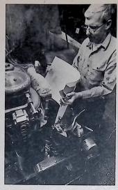
When the metal has hardened, the stereotype plate is a mirror-image replica of the mat. After being trimmed, the plate is marked with a page number and it travels on a kind of moving sidewalk to the correct press.
