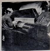
Because the presses move fast, they use paper very rapidly. Newsprint is moved via an underground tunnel from the Tribune's newsprint warehouse on the Chicago River to the reelroom where the rolls are prepared for use.
