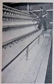
At the mill, logs are ground into pulp and mixed with water and chemicals. The resulting mixture is poured onto a screen and the water drained off, leaving a thin wet sheet. Giant hot rollers press and dry the wet pulp as it moves thru the paper-making machinery. When dried, pressed pulp emerges as newsprint and is wound onto a roll weighing several tons. This roll is cut into smaller rolls to fit the presses. A five foot wide roll weighs about 1,700 pounds and contains six miles of paper.
